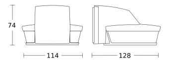
Possible mounting height: 2,00 m - 5,00 m Orange: radial Black: tangential 3 scalable zones
